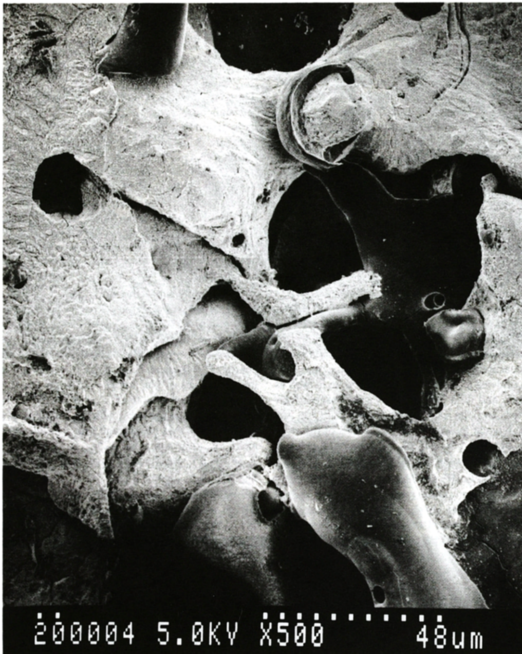
FIG. 4(b). Scanning electron microscope photograph of an exemplary thermal spray coating: self-bonding aluminum bronze copper aluminum with a porous substrate thickness of 25.4 \mu\text{m}
